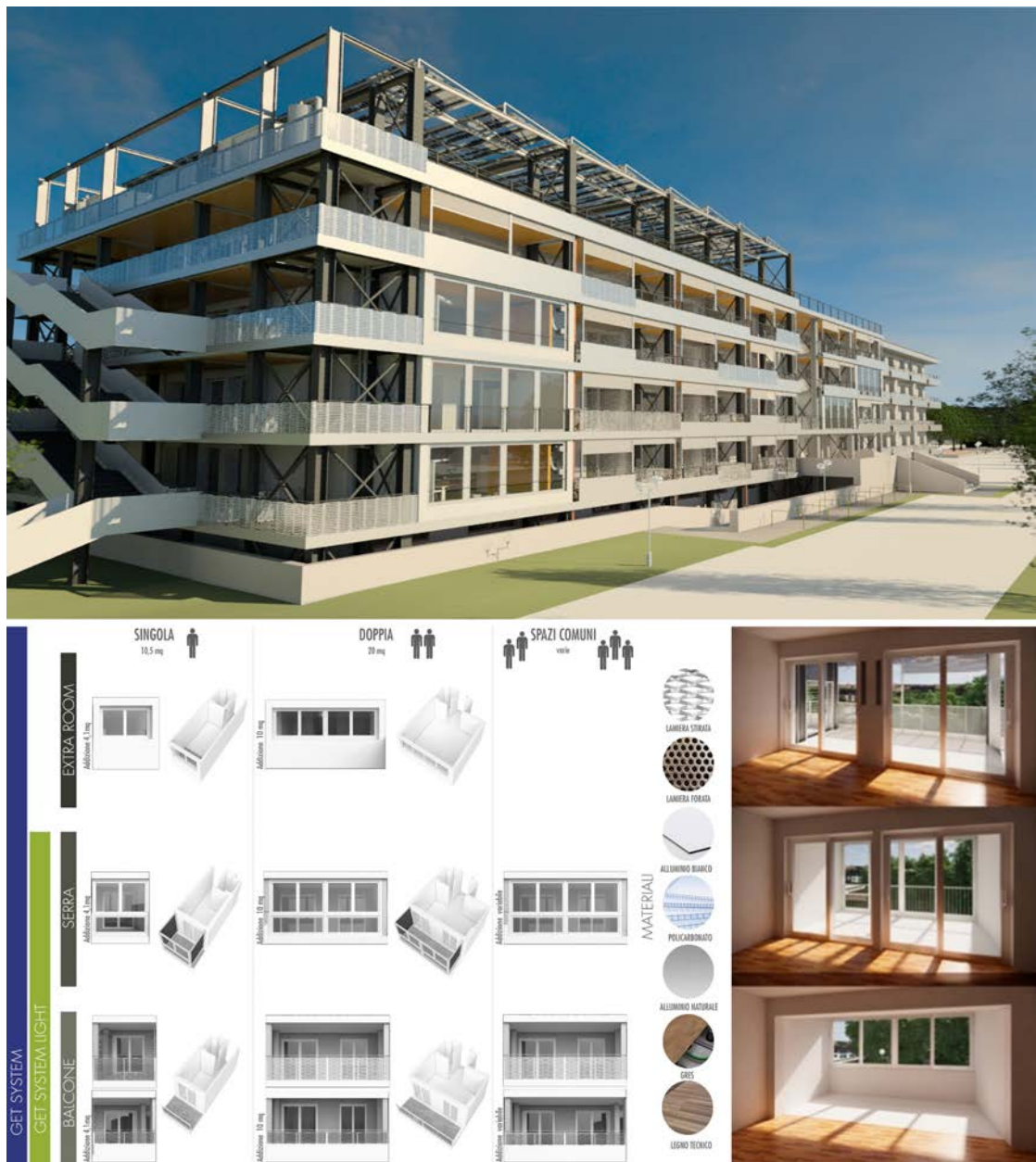
Figure 5. Top: a view for the construction of the new facade and the reshape of the students' house in Zografou, Athens (© 2021, "Pro-GET-one" team, BIM Models by M. Iannantuono and V. Giannakoupoulos). Bottom: abacus of the different Add-ons solutions, customizable in function of the specific design requirements (left) (© 2018, Cinti, A.); views from the inside of the added volumes (right) (© 2021, M. Iannantuono).
