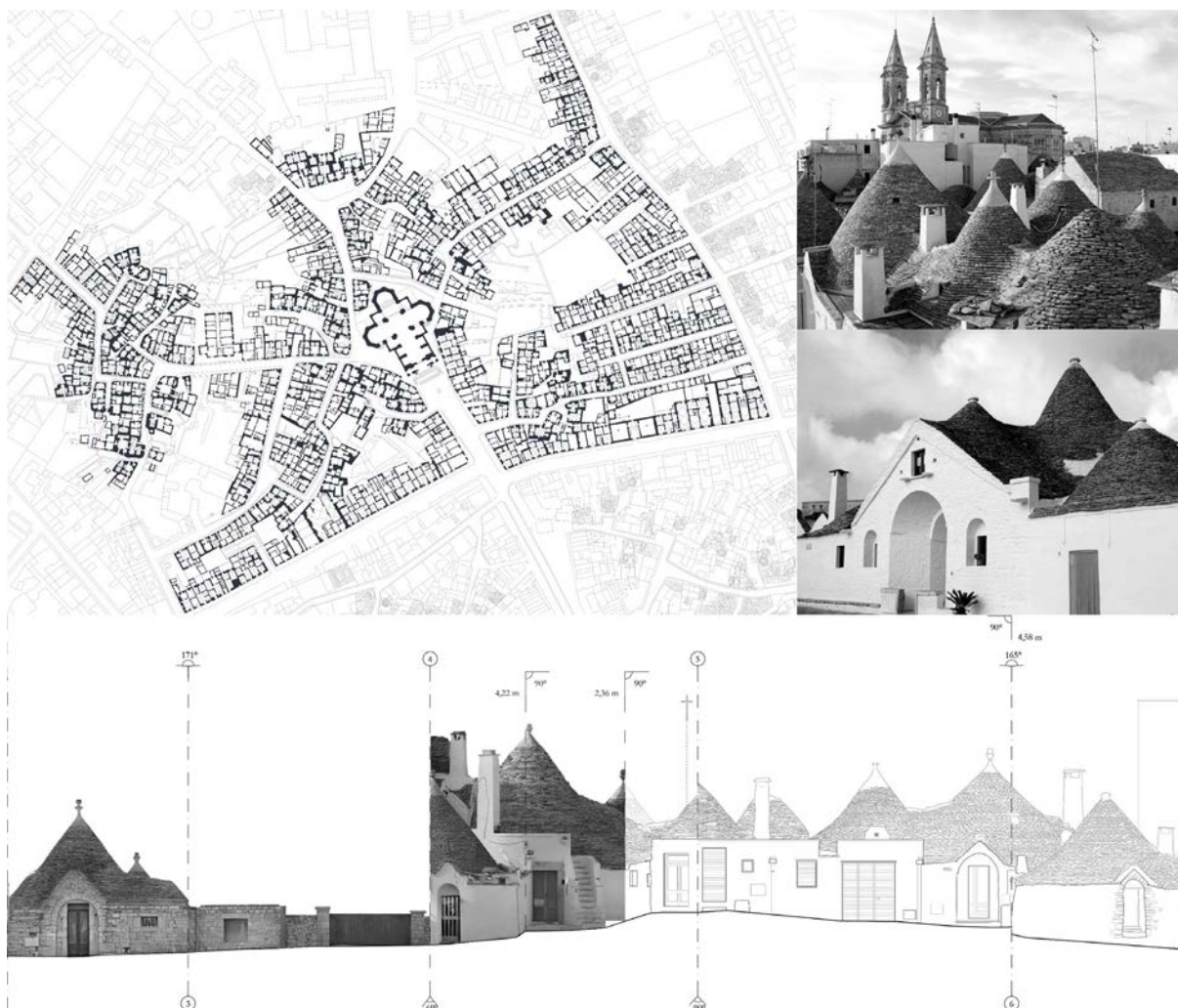
Figure 3. Planimetric assembly, photogrammetric survey and redraw of urban fronts.
